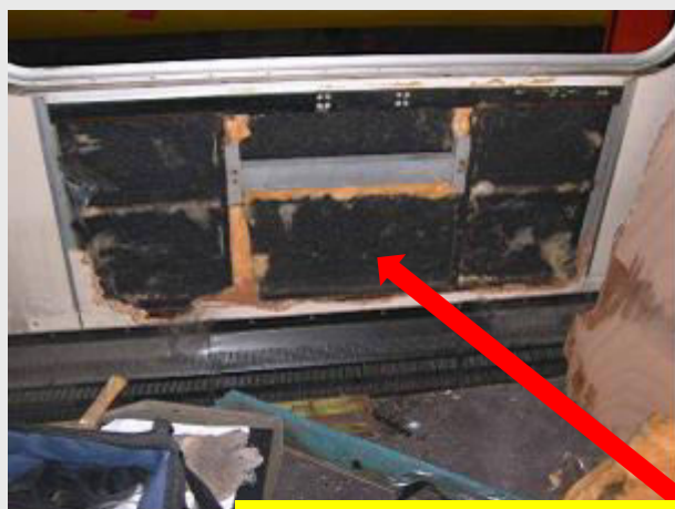
Walls coating (bitumen coating to main steel walls of train)
