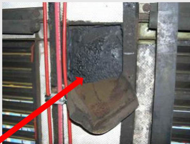
Walls coating (bitumen coating to main steel walls of train)
